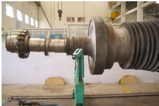
Before bend removal (103mm bend)
