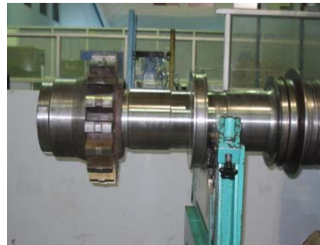
After bend Removal
