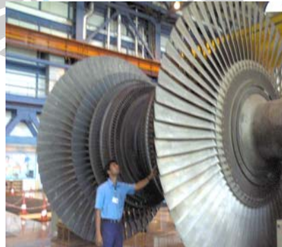
500 MW Turbine Rotor
