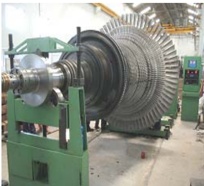
25 MW Turbine Rotor
