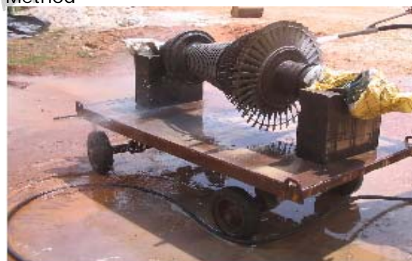
High Pressure water - jet cleaning of Turbine Rotor
