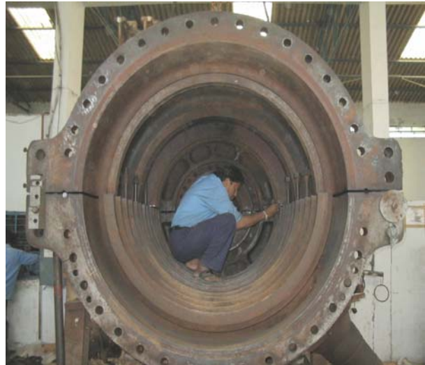
Casing Parting plane clearance checking
