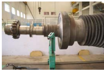
Before bend removal (103mm bend)
