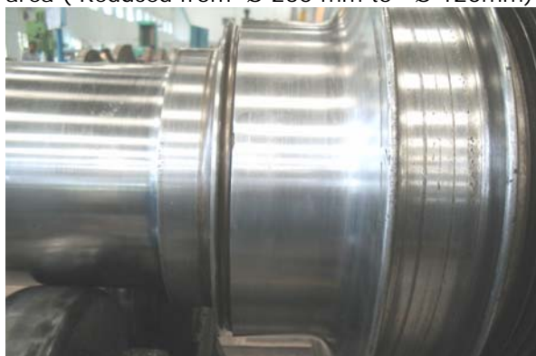
After repair ( Restored to \text{\O} 250 \text{ mm} )
