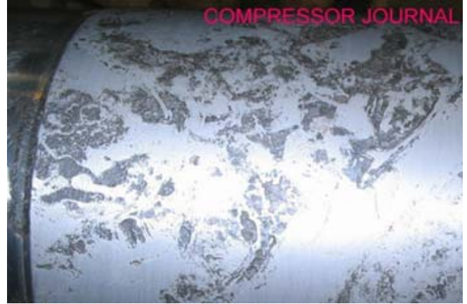
Compressor Journal before metal build up.
