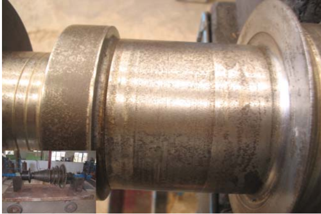
Turbine Journal before metal build up.
