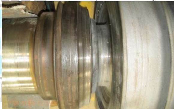
Gland after metal build up and machining
