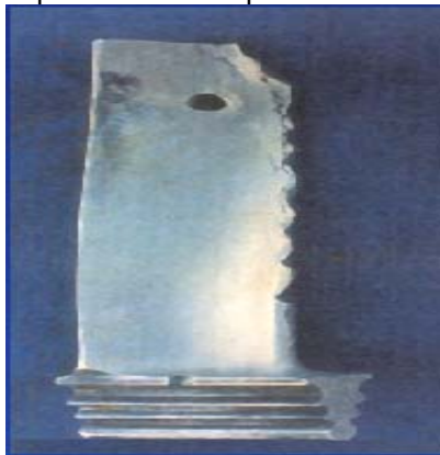
Eroded Blade in Received condition
