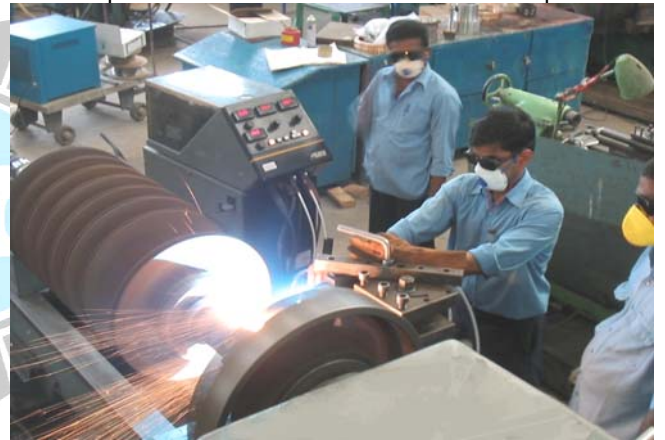
Metal spray on Compressor Journal ( Wire Arc Spray)
