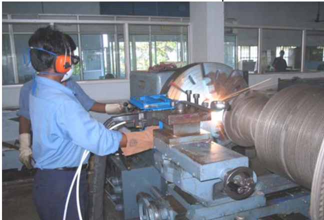
Metal spray on Turbine Journal ( Wire Arc Spray)
