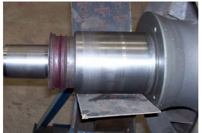
After metal build-up and machining
