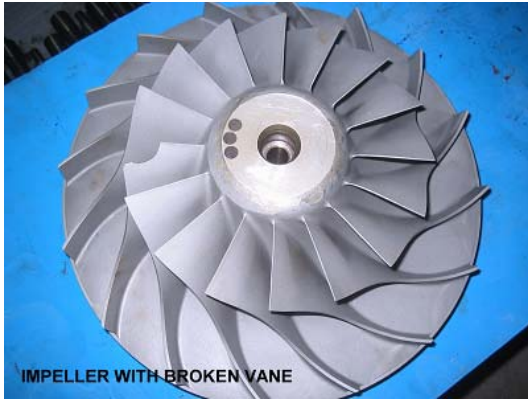
Impeller with Broken vane
