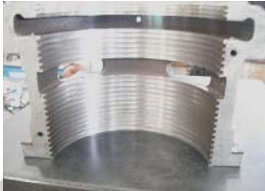
Gland after metal build up and machining
